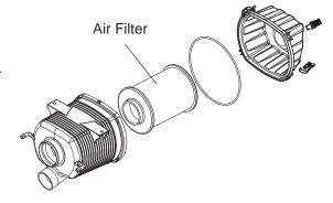
Inspect the air box for oil or water deposits. If present, drain into a suitable container.
